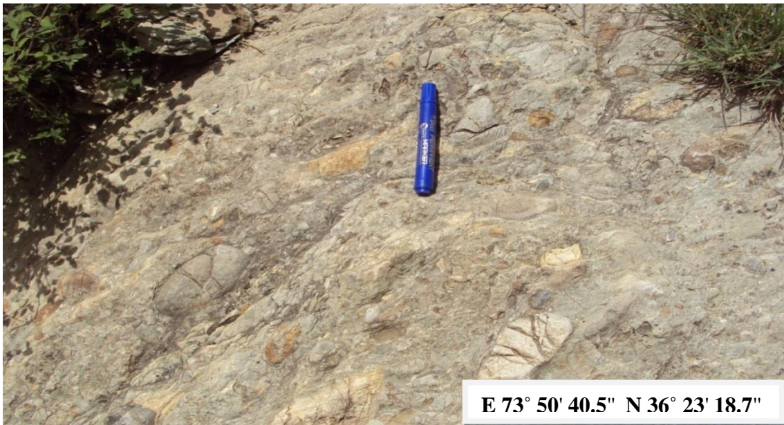
Fig.3.6. This photograph showing brecciation in the BASD volcanics along local faults/shear zone.
